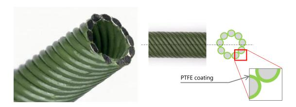
By forming PTFE precoated fine wires, fully coated each filar add excellent lubricity to both inside and outside of cable without losing the property of the cable. This processing applied to one layer hollow cable like ACT ONE or Wire coil. Ideal for applications requires lubricity and chemical resistance in addition to the property of the hollow cable like 1 to 1 Torque response and flexibility.
