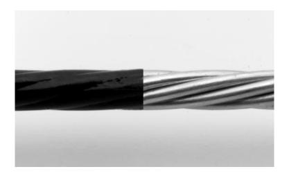
A stainless steel cable assembly may be sprayed, dipped, or extruded with PTFE, Nylon, and other coatings for your particular abrasion-resistance, lubricity, low coefficient of friction, and long-term durability requirements. Asahi Intecc can precisely mask the ends of the coated stainless steel cable assemblies to attach various in-house iron (FE), stainless steel (SUS, SS), Aluminum (AL), Copper (Cu), and other metallic finishes.
